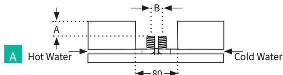
Prepare the input pipes as per diagram.
