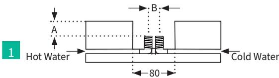
1 Prepare the input pipes as per diagram.
