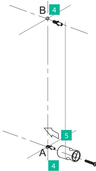
4. Push wall anchors into holes.
