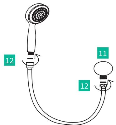
11. Attach the supply elbow to the supply connection on the wall.
