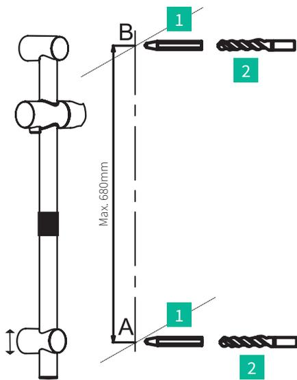
The bottom bracket can be adjusted to desired height
