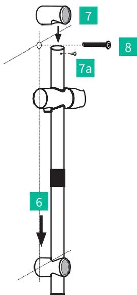
6. Slide the rail tube through the bottom bracket.
